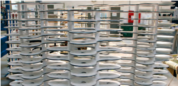
Special RSiC setters with coating for firing porcelain.
