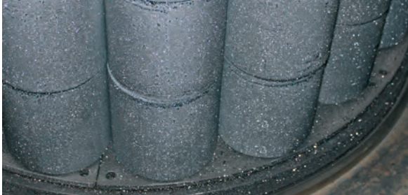
Triangular RSiC bottom plates for SiC firings - provides excellent homogenous heat distribution throughout the parts.
